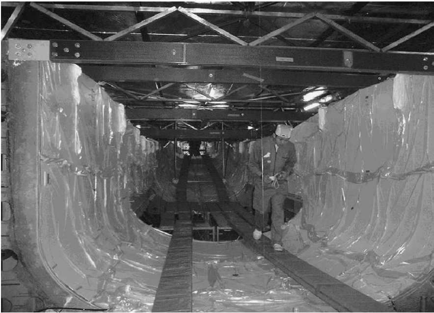
Figure 14. Debulking of upper fuselage part.
