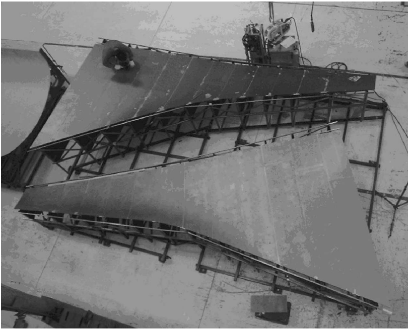
Figure 8. Lay-up tool of wing cover.
